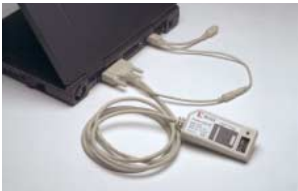
Figure 7: Laptop PC IV Cable Connection
